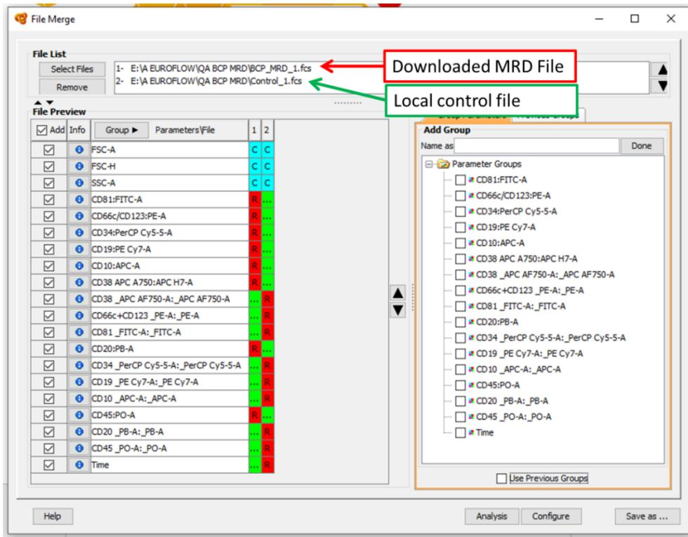
If necessary, group the parameters so that all the parameters are marked with “C” as “common”.
